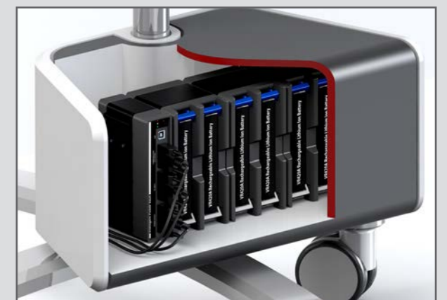
536Wh 'IPV06' installed in a medical workstation
