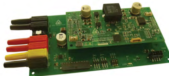
CHARGER MODULE (50ABB002) MOUNTED ON EVALUATION MODULE (EVAL008)
